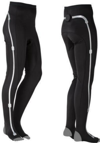
**Figure 12.** The e-skin smart pants from Xenoma including a seven MIMU sensor network.<sup>1</sup>
