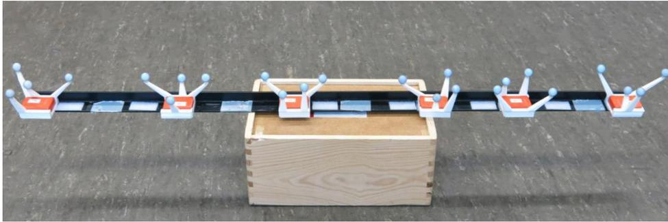
**Figure 17.** The MIMUs inserted in the corresponding RBs necessary for the lower body motion analysis. The RBs are mounted on a rigid stick. The stick was moved around all three spatial axes during the record.
