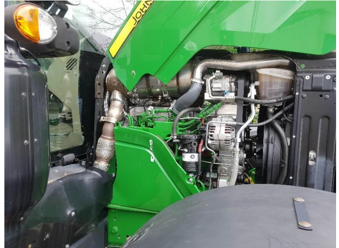
FIGURE 34: HDMK ENGINE INTEGRATED INTO THE JD TRACTOR
