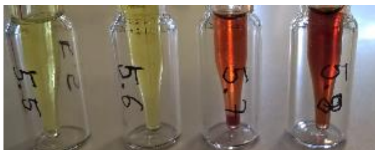
Figure 4-12: Reaction of vanillin with NAcDAP in 60 % technical ethanol after 24 h incubation time. Reaction preparations depending on the incubation time (from left: room temperature, 40 °C; 75 °C and 100 °C).
