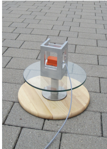
Figure 4.3.: A high precision aluminum cube on a turntable made of glass and aluminum with a flat wooden plate as a levelled base served as test setup for performing known motions. Here, the Xsens MTi is mounted inside the cube.
