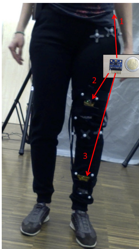
Figure 4.15.: Test setup. The red arrows show three IMUs which are mounted on 1.pelvis (not visible), 2.upper leg and 3.lower leg
