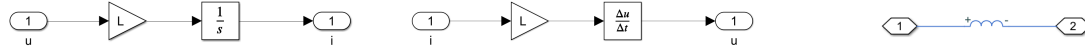
(a) Causal inductance model u/i (b) Causal inductance model i/u (c) Acausal inductance model
