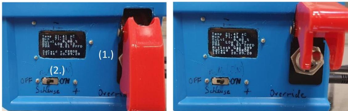
**Fig. 7: Operator control interface with the Killswitch (1) and Slide Switch (2) disengaged (left) and engaged (right). Note the change in the OLED display line 6.**
