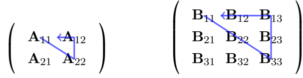
Fig. 3.1: For the Mandel notation the main diagonal of the matrix is traversed first before moving upwards in the column. In the three-dimensional case one additionally moves back to the start along the first row.
