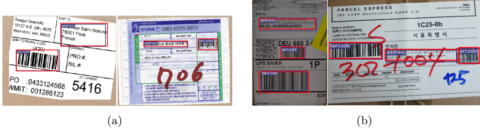
Figure 6.7: Examples of detected barcode and address areas (a) on generated images and (b) on the real dataset: red boxes are ground truth, and blue boxes are detected regions
