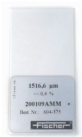
Figure 4.7: Acrylic sample of a thickness of 1.5166 mm \pm 0.4%
