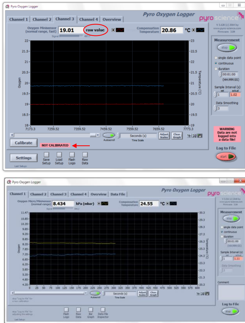
Figure 111 Example of the graphs obtained from the oxygen meter readings before (top) and after (bottom) calibration.
