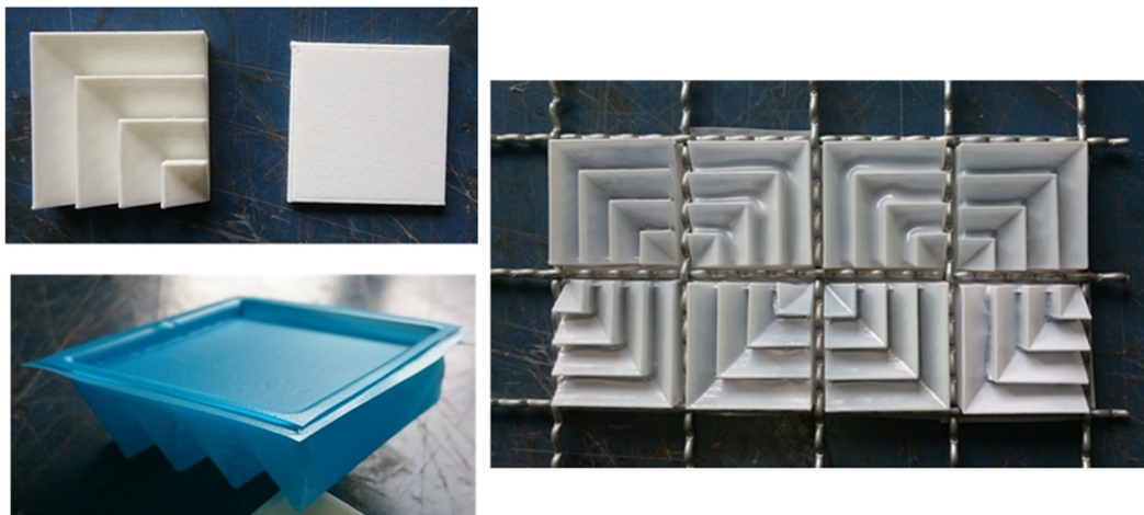
Figure 5. Molded recycled plastic forms that act as PCM containers for ceiling construction [39].
