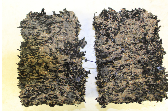
Figure 60: Sand S2 at 30% chips content after cyclic test
