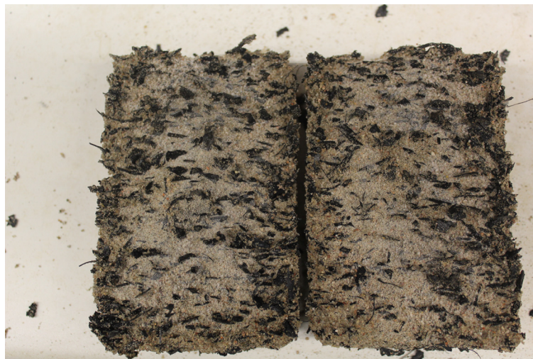
Figure 59: Sand S2 at 30% chips content before test
