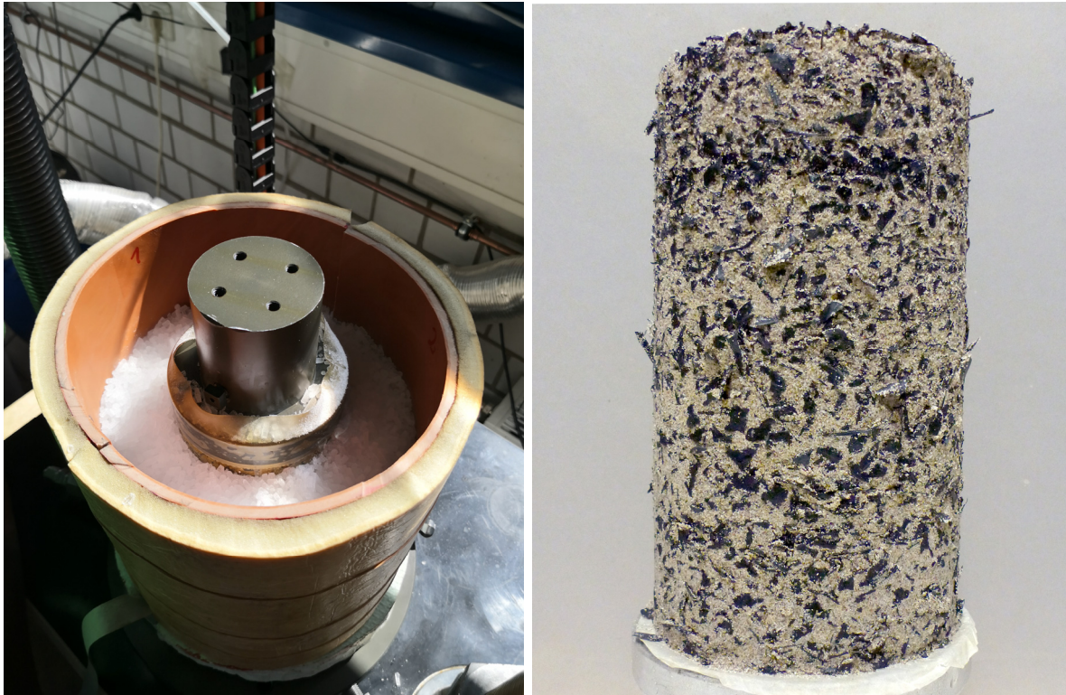
Figure 58: Sample freezing left dry ice and right a two days frozen sample in freezer after sample preparation
