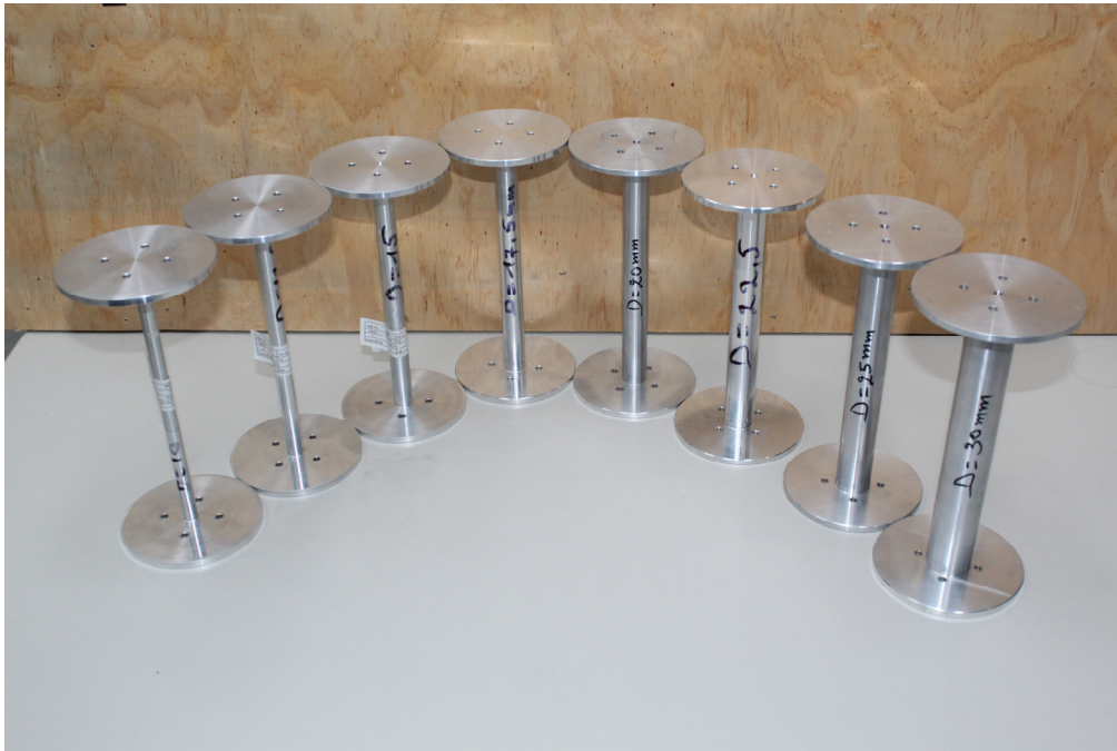
Figure 63: Various aluminium calibration bars used for the calibration
