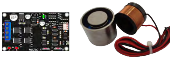
Figure 7.4: Voice-coil motor and motor driver
