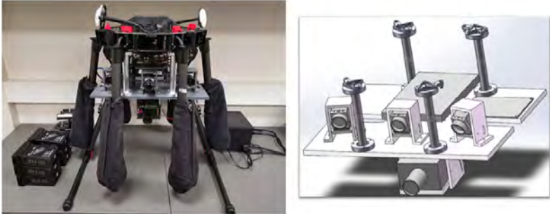
Figure 1.2: Measurement platform for 3D reconstruction attached to an UAV [68]
