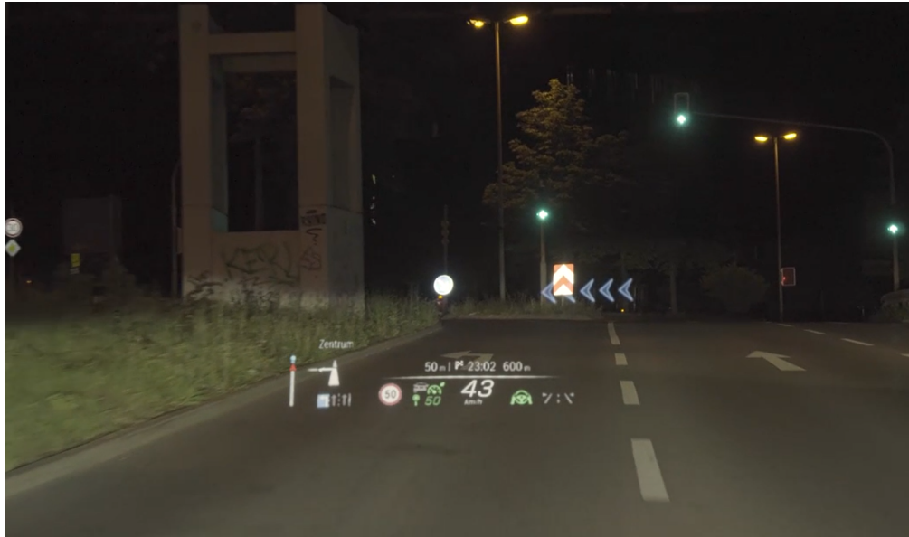
Figure 2.3: AR head up display of the Mercedes S-Class [28].
