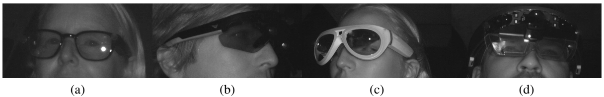
Figure 6.3: Example, cropped IR images of all four glasses in the recordings: (a) North Focals Generation 1, (b) EverySight Raptor, (c) Mini Augmented Vision (d) Microsoft HoloLens 1.
