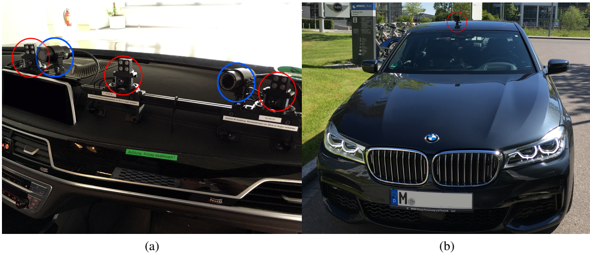
Figure 6.1: The hardware setup on the dashboard inside the car and the car itself used for the dataset recording. (a) There are three infrared cameras with flashers on top for the image recording (red). Two marker-based cameras acquire the 6-DoF ground truth poses (blue). (b) The dataset was recorded in a 7 series BMW, here on top with the utilized 360° camera (red) to acquire footage for simulation to be used during recording.
