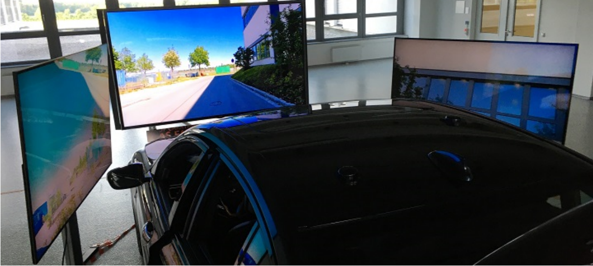
Figure 6.4: The simulation setup. A route is played which was prerecorded with 360° camera and edited accordingly for the three screens.
