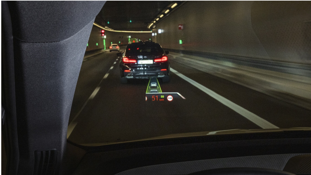
Figure 2.2: Head up display of the BMW iX [27].
