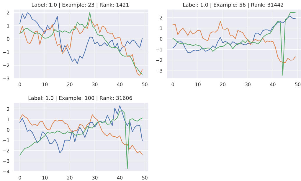
Figure 9.6: All samples are anomalies within the ground truth, but their labels were flipped during the training. Only sample 100 was successfully identified as mislabel by the loss-based approach.
