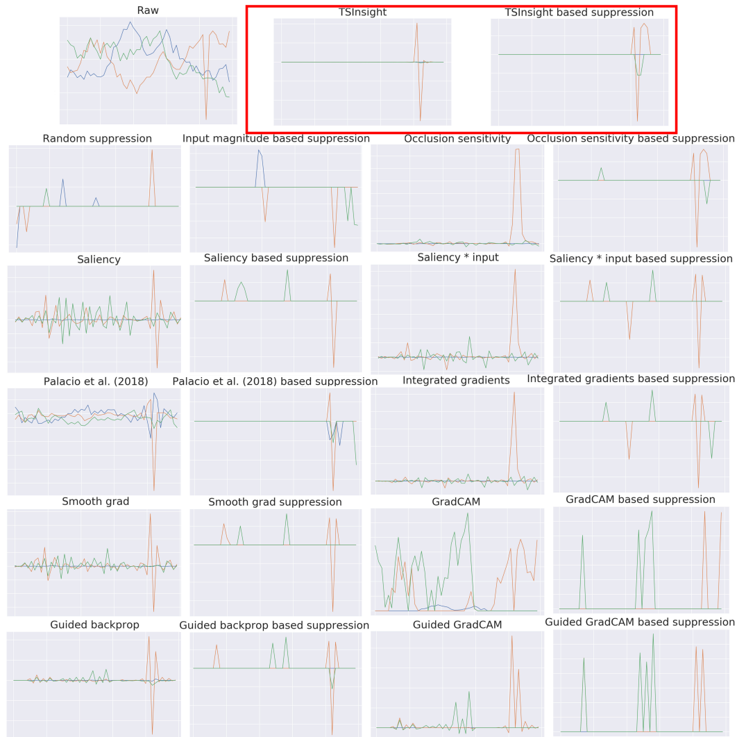
Figure 8.5: Output from different attribution methods as well as the input after suppressing all the points except the top 5% highlighted by the corresponding attribution method on an anomalous example from the Synthetic Anomaly Detection dataset (best viewed digitally). All methods were able to correctly identify the anomalous spike given the simplicity of this dataset. However, qualitative differences exist between different methods.
