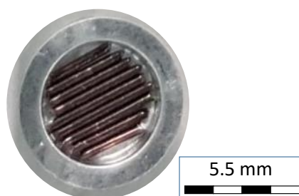
Figure 7.1: Sample pan for DSC measurement filled with SMA wire sections to achieve high pan coverage.
