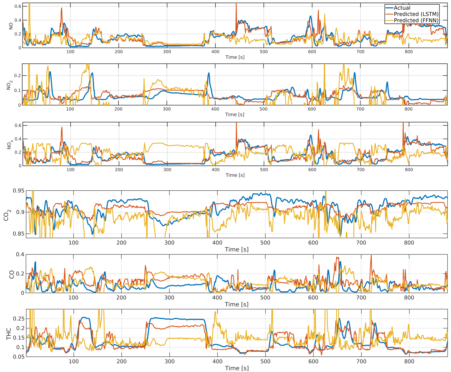
Figure 11: Emission prediction results with LSTM and FFNN. All pollutants are drawn on a unitless and normalized scale between 0 and 1.
