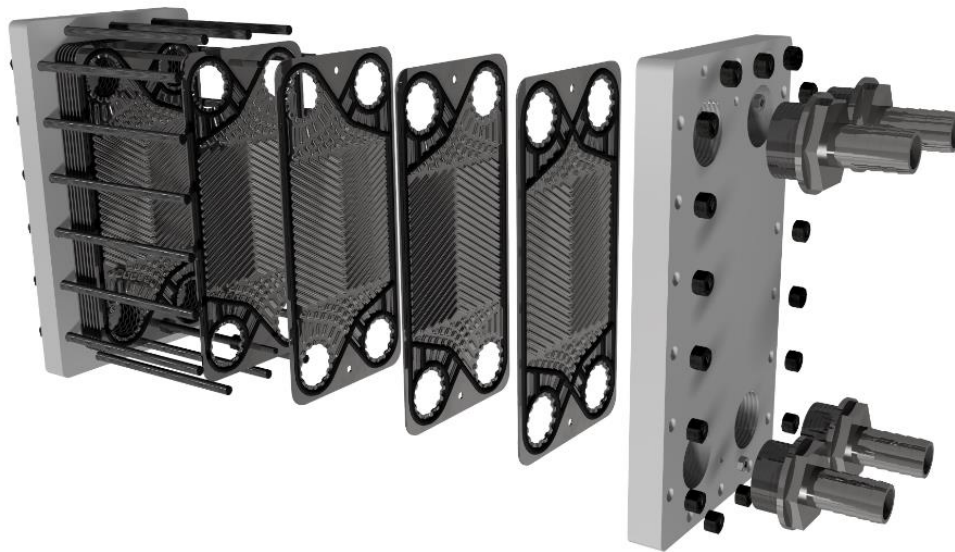
Fig. 3.6: Exploded view of the developed heat exchanger.
