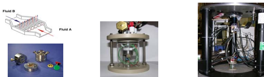
Figure 2: Left: Micro mixer from IMM, Mainz, Germany; Middle: Micro mixer with housing for thermostatzation; Right: Complete installation of micro mixer with NMR probe under the NMR magnet
