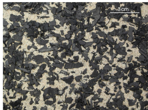
Fig. 2 Medium sand S2 mixed with rubber chips at 20% chips
