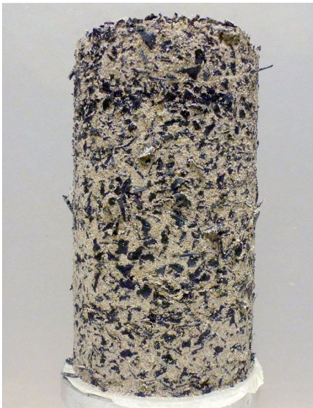
Fig. 4 Test specimen stabilized by dry-ice freezing for the sake of visualization (Banzibaganye and Vrettos, 2022)
