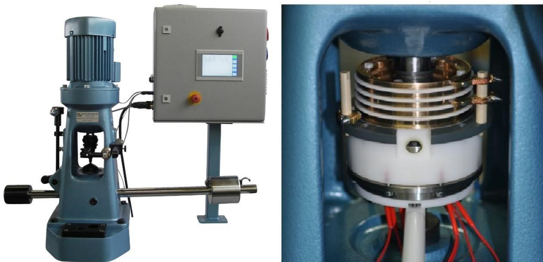
Figure 4.1: Test bench for the experimental investigations: a) Four-ball-tester [HP19]; b) GESA cell installed in the four-ball-tester [Bec20]
