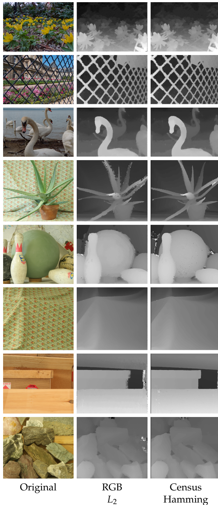
FIGURE 5.17: Qualitative results for real-world scenes with different comparison function for matching cost construction: first three rows – EPFL dataset from [127], the rest – Middlebury dataset [54, 133].
