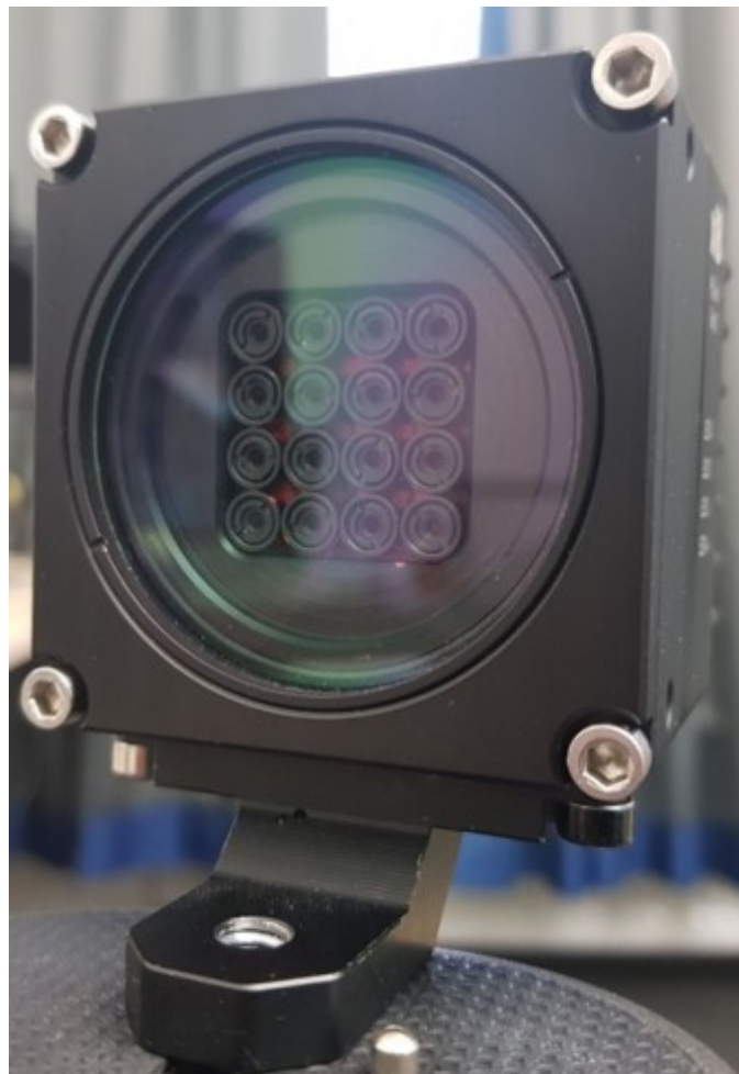
FIGURE 2.17: A LF capturing device, consisting of single RGB camera with 4x4 lens array in front of the image sensor
