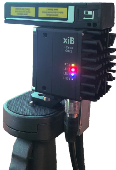
FIGURE 6.5: Setup of the distance measurement device on top of the used LF camera
