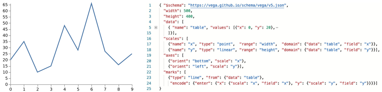
Figure 2: Line chart created using Vega: the Vega code (right) describes the relevant syntactic components of a line chart (left).
