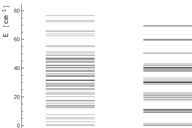
Figure 4. Energy of the 108 low lying micro-states of \text{Os}_2\text{Ni}_3 from spin Hamiltonian calculations (scaled CASOCI parameters). Left: all spin Hamiltonian parameters included, right: Ni single-ion \mathbf{D} tensors set to zero.
