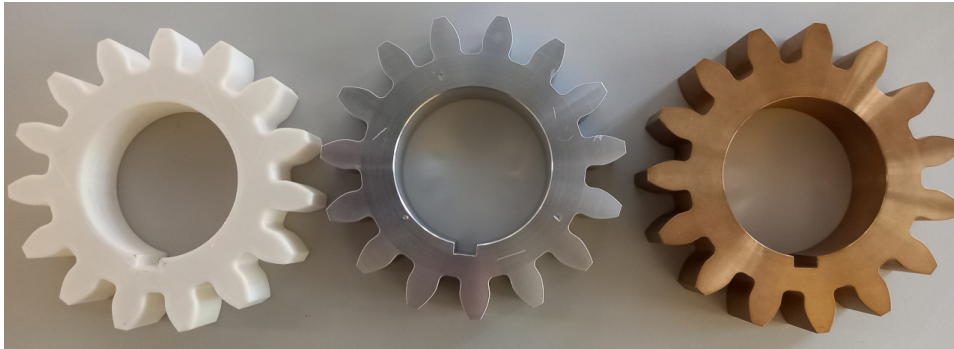
Figure 1.1: Inspected parts with the same geometry but different reflectance and texture appear significantly different.
