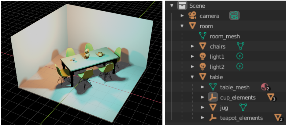
Figure 2.3: Example of a scene graph. The scene represents the root node where the camera and room are its children. Further, the room has a table for child which has cup, jug, teapot for children.
