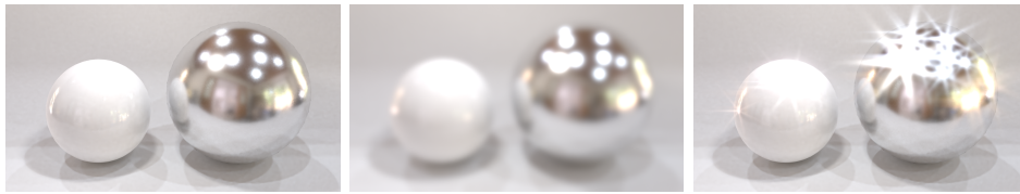
Figure 2.45: Left: rendered image. Middle: blur post-processing. Right: glare effects post processing.
