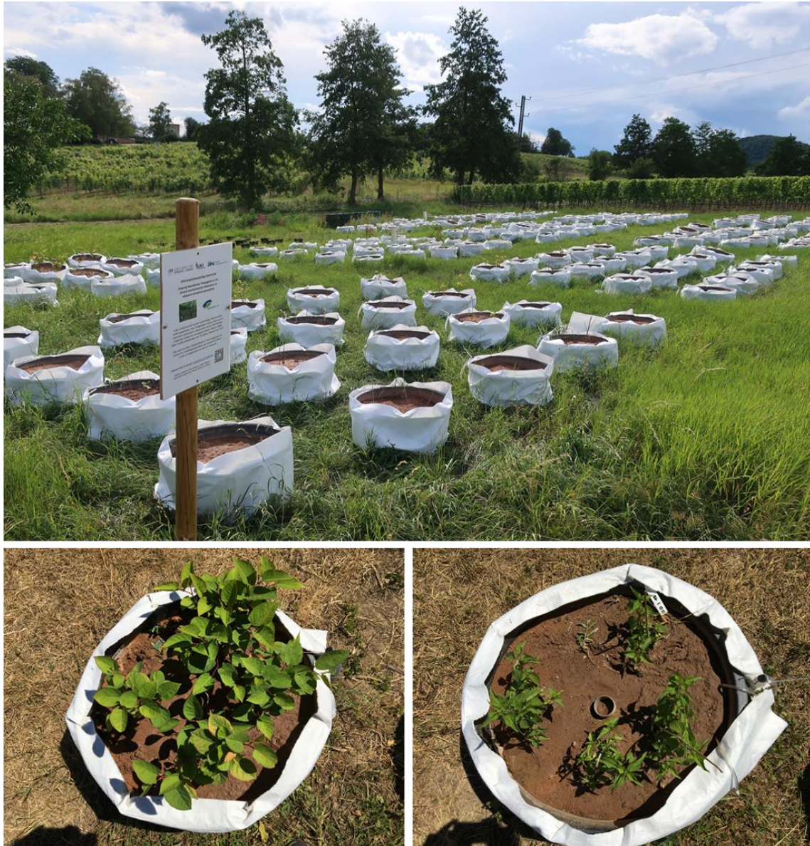
Fig. 2 Experimental setup of the experiment. General view of the pots arranged in a randomized block design and sample pictures of Fallopia japonica (left) and Urtica dioica (right) growing in the pots in spring 2021. From Schmitz et al. 2023, see Amendment II.
