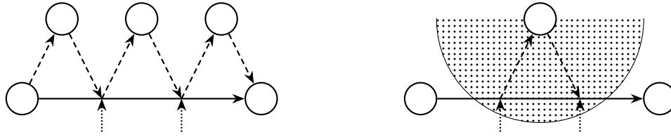
Figure 2.3.1: The paths of the truck and drone are shown using solid and dashed lines, respectively. The dotted arrows on the solid arcs indicate locations at which en route operations are possible. On the left-hand side, one fast-moving drone is able to perform multiple operations during a single transition of the truck. On the right-hand side, we assume that the customer might only be served by drone, if the drone is launched and retrieved within the feasible region (indicated by the dotted pattern). Here, through en route operations, a drone is able to perform an operation that would otherwise not be possible.
