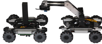
(b) Cart and carrier meet at a suitable position and exchange the object
