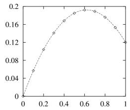
Figure 3: Velocity profile for Couette flow
