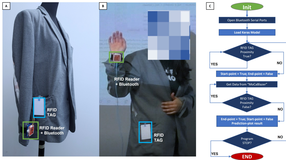
Figure 4.6.: Real-Time Recognition System. A The "MoCaBlazer" with the RFID Reader-Tag Pair Positions. B Volunteer Wearing the "MoCaBlazer" with the RFID Synchronization System. C Flow Diagram of the Real-Time Recognition Python Script.
