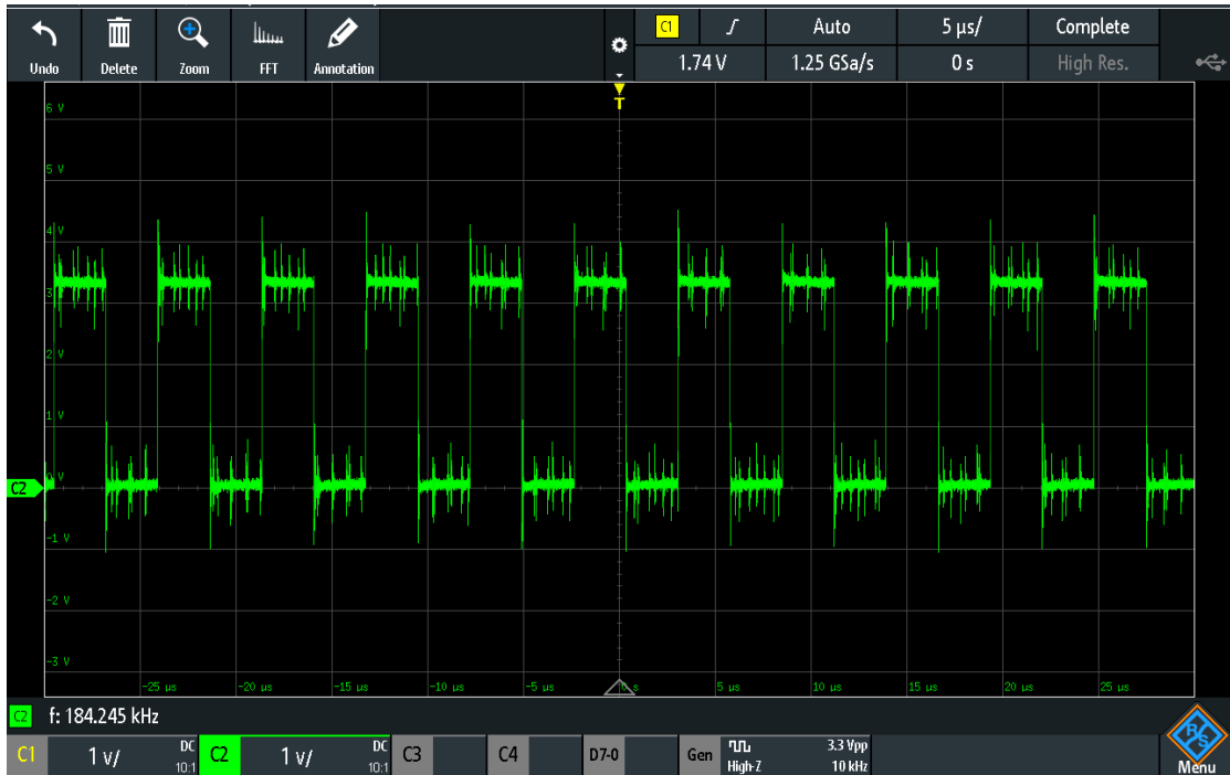
Figure 5.39: The output from non-intrusive sensor1 using one of the extrinsic patterns at typical operation condition: T = 24^{\circ}\text{C} and V_{DD} = 3.3\text{ V} .
