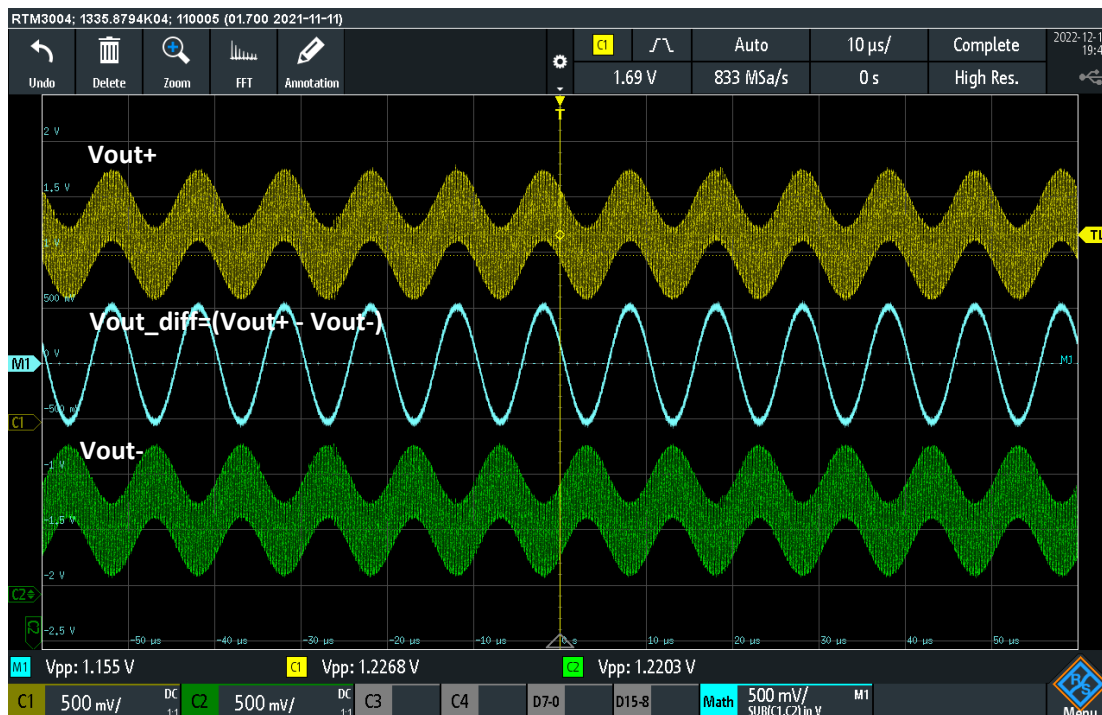
Figure 4.11: The transient response of the output to the fully differential sinusoidal input signal under unstable conditions.
