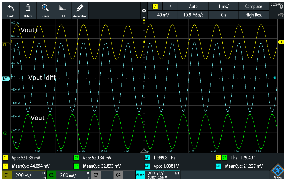
Figure 4.34: Sinusoidal transient response of the filter
