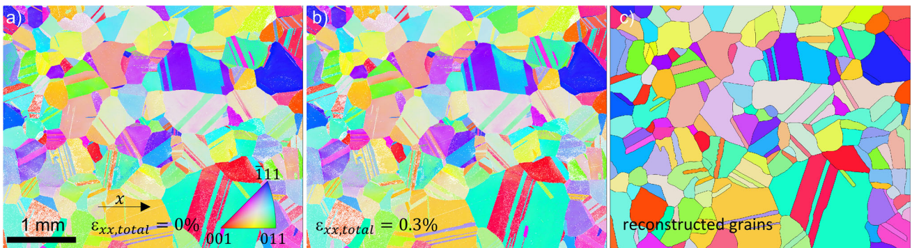
Figure 9 EBSD data at a \epsilon_{xx} = 0\% , b \epsilon_{xx} = 0.3\% and c reconstructed grain structure of sample 2.
