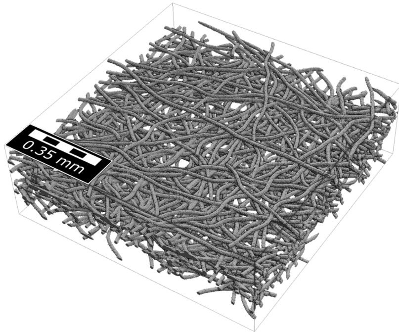
Figure 2.6.: Generated validation structure 3 with a solid volume percentage of 11.9% and 339 individual fibers.
