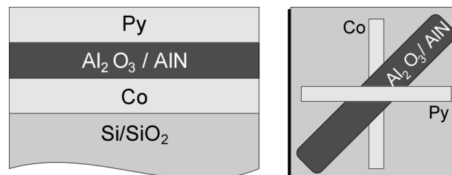
Fig. 1 : Schematic view of a patterned TMR junction. The layer thickness of Co and Py is 150 Å each. The barrier layer varies from 20 to 40 Å.
