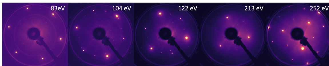
Figure (2.1) LEED images of the pristine Ni(111) surface. In addition to the clear Ni(111) spots, residual carbon contamination is visible. The images were acquired at electron beam energies of 83 eV, 104 eV, 122 eV, 213 eV and 252 eV.
