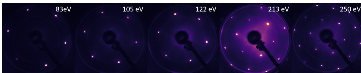
Figure (2.2) LEED images of the graphene/Ni(111) surface. A clear six-fold symmetry, typical for graphene is visible. The graphene spots coincide with the Ni(111) spots. Therefore no additional spots are visible. It is noteworthy to mention here, that the residual carbon clusters from the Ni(111) surface were condensation centres for the graphene-sheet formation, therefore these spots are no longer visible. The images were taken at 83 eV, 104 eV, 122 eV, 213 eV and 252 eV electron beam energy.
