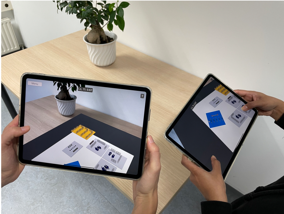
Figure 6.10: Conceptual FLP with the multi-user MR-HHD app: A factory layout is collaboratively optimized by manipulating factory units using Move'n'Hold : The left user uses translation through direct mapping (left-thumb-touch only) whereas the right user applies continuous rotation (left-thumb-touch and right-thumb-touch).
