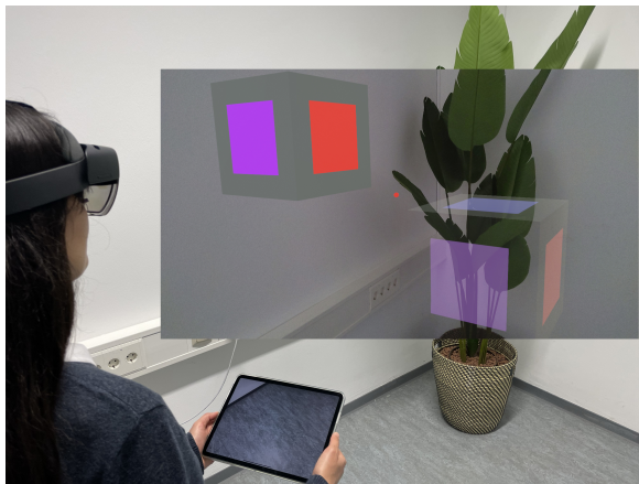
(b) Example MR-HMD: Selecting an object by hovering it with the red point while no touch is applied on the tablet controller.
