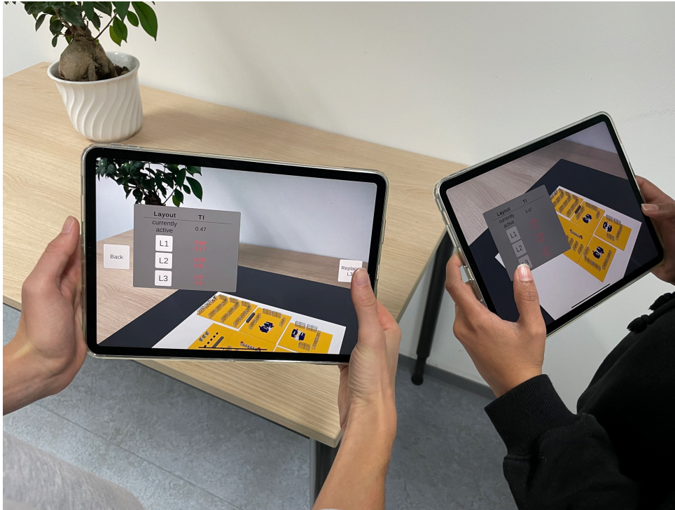
Figure 6.12: Conceptual planning with the multi-user MR-HHD app: The currently active layout is saved by replacing the layout with the worst transportation intensity.
