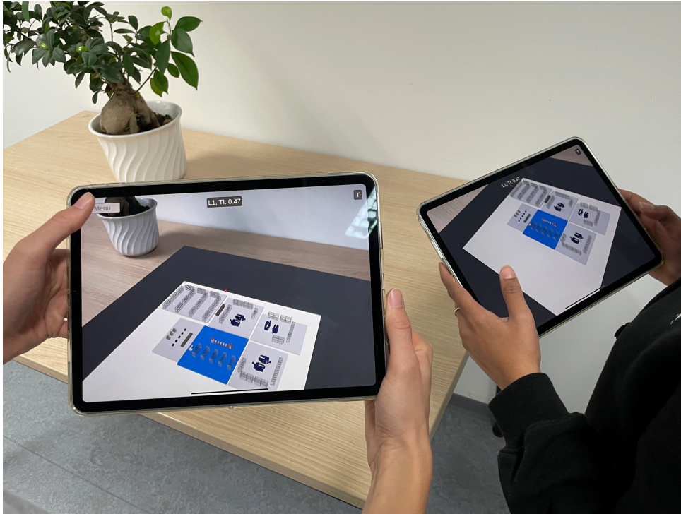
Figure 6.11: Conceptual FLP with the multi-user MR-HHD app: To compare the currently active layout against other layouts, the host opens the menu by clicking the respective button.
