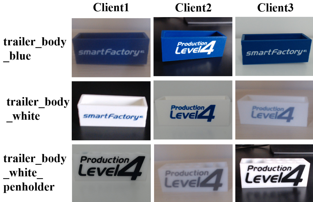
Figure 3.16: Federated Ensemble Trailer Dataset: Centralized trailer dataset divided randomly across 3 clients for FL experiments.
