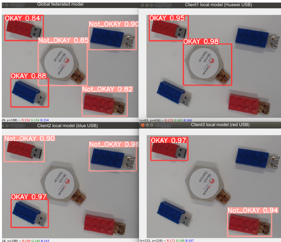
Figure 4.11: Live inference comparison of the global federated model (top left) against local client models: Client1 (top right), Client2 (bottom left), and Client3 (bottom right). The federated model successfully detects and classifies all USBs, including previously unseen variants, whereas local models show misclassifications and limited generalization. Confidence threshold = 0.20.
