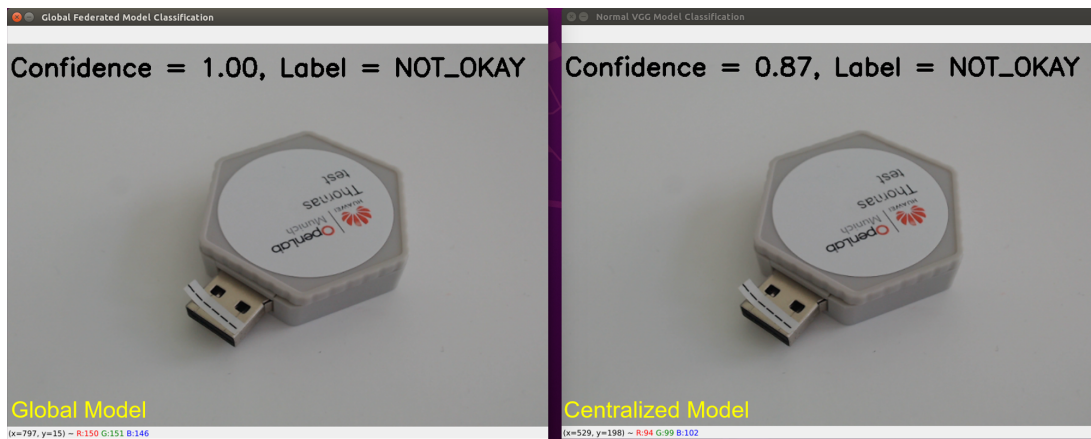
Figure 4.5: Live inference on a Client1 USB stick using the global federated model and a centralized VGG-19 model. The ground truth is NOT_OKAY. Both models classify correctly, but the federated model achieves higher confidence, illustrating its stronger reliability under deployment conditions.
