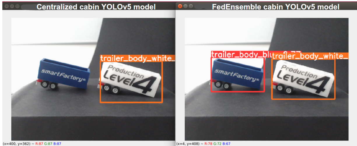
Figure 4.18: Live inference comparison between centralized YOLOv5 (left) and FedEnsemble YOLOv5 (right) on trailer detection (Confidence Threshold = 0.20). The centralized model fails to detect class 1 and produces an imprecise bounding box for class 2, whereas the FedEnsemble model correctly identifies and localizes all trailer types with precise bounding boxes.
