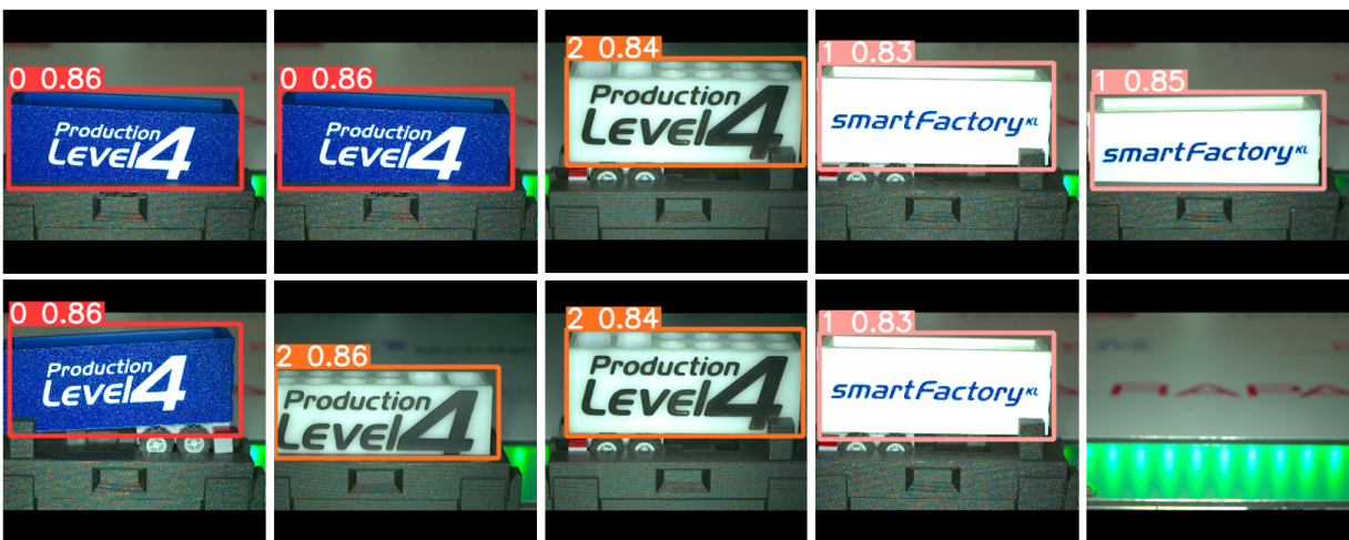
Figure 4.20: FedEnsemble YOLOv5 model inference on SmartFactory-KL demonstrator images. All trailers are detected with accurate bounding boxes and no false positives on background structures (Confidence Threshold = 0.20).
