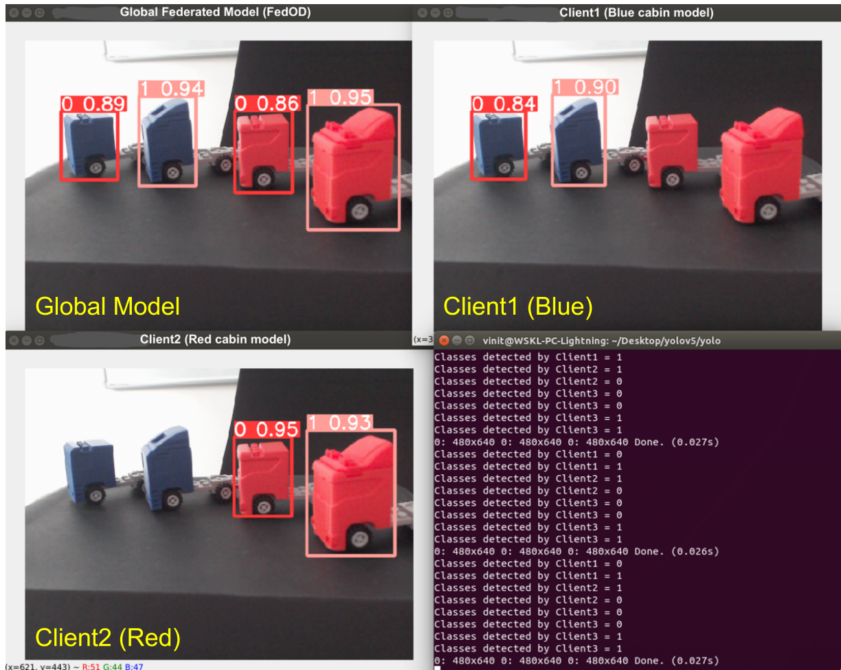
Figure 4.13: Live inference on mixed cabin types using Client 1, Client 2, and Global FedOD models (Confidence threshold = 0.20). The federated model detects both cabins with precise bounding boxes and high confidence, while local models detect only their respective cabin types and fail on unseen geometries.
