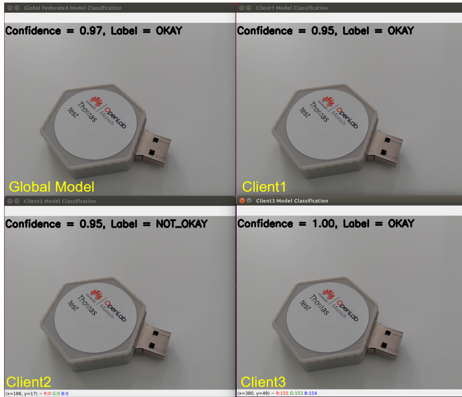
Figure 4.1: Live inference on a Client1 USB stick using the global federated model and client models trained on their respective local datasets. Ground truth: OKAY.
