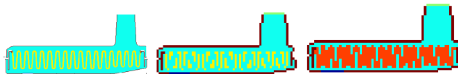
Figure 12: Pleats in the filter on different grids. Fine grid resolves the geometrical shape of the filter and the pleats, where as the coarse grid does not. Subgrid treats all pleats as a block of filtering medium with upscaled permeability computed using fine scale algorithm.
