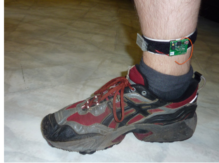
Fig. 4. Real-world AAL experiment: Floorplan and placed nodes in the flat; M.: PIR movement detector; D.: Door sensor (reedswitch and magnet); a tenth, mobile node, is not shown Fig. 5. Real-world sport experiment: AmICA node and a lithium polymer battery mounted on a athlete's leg
