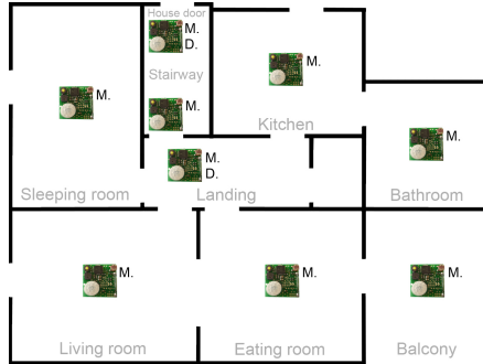
Fig. 4. Real-world AAL experiment: Floorplan and placed nodes in the flat; M.: PIR movement detector; D.: Door sensor (reedswitch and magnet); a tenth, mobile node, is not shown Fig. 5. Real-world sport experiment: AmICA node and a lithium polymer battery mounted on a athlete's leg
