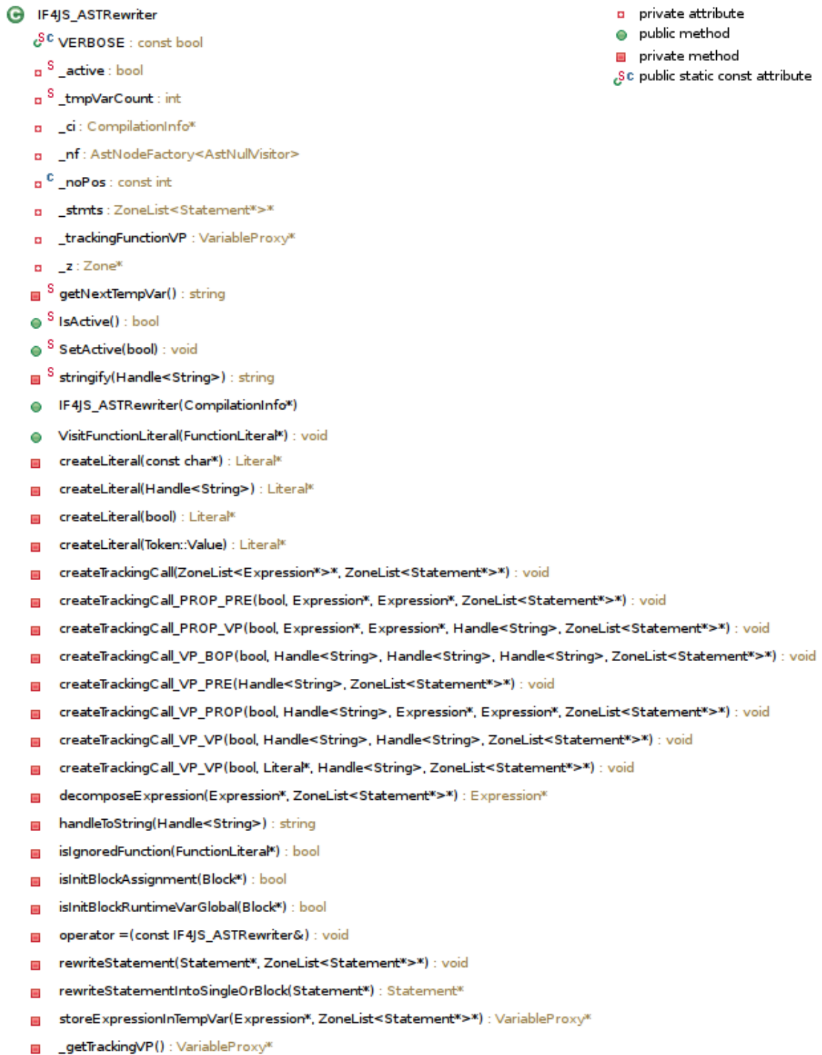
Figure 5.2: The structure of IF4JS_ASTRewriter . The S indicates static members.
