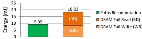
Figure 5.3: Energy required to read and write the paths from DRAM is two times as high as recomputing it on the FPGA alongside the later part of the Longstaff-Schwartz algorithm.
