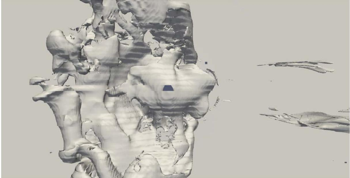
Figure 2.1: An isocontour produced on the yA31 data set with 128 processing cores and no ghost cells, there are clearly visible holes in the isocontour and seams are also visible in areas with high gradient.
