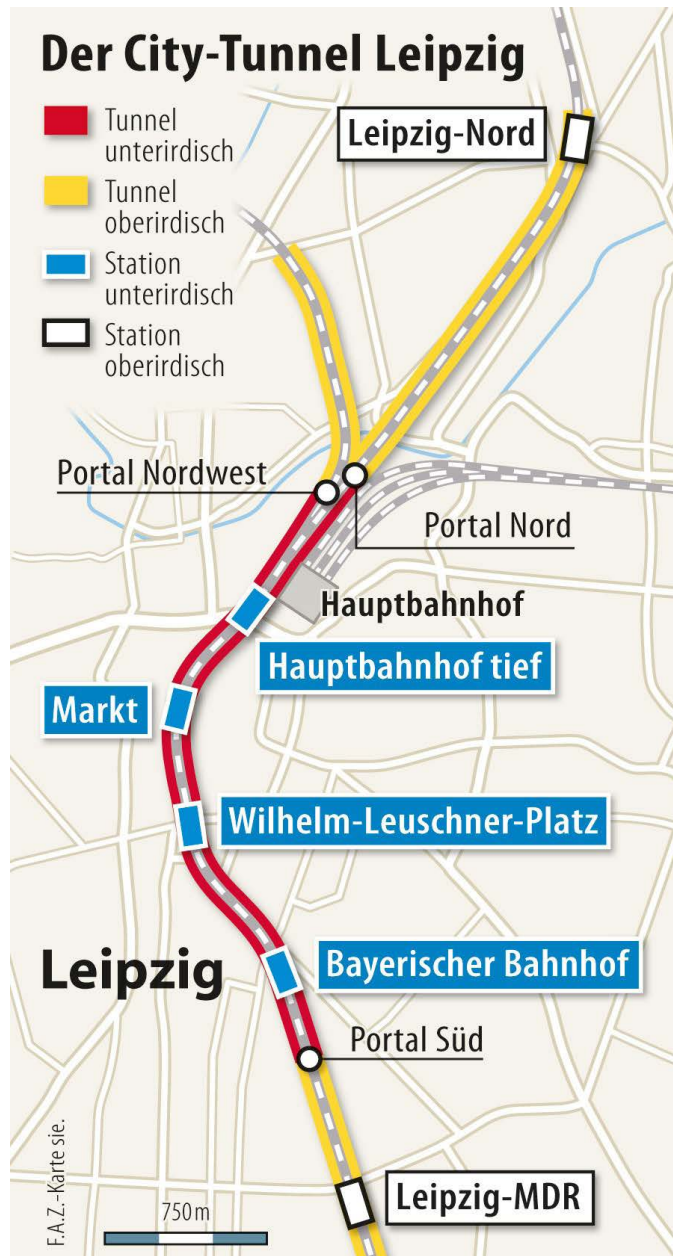
Map 6.11: Leipzig City Tunnel as part of the broader S-Bahn Network. Source: https://www.faz.net/aktuell/wirtschaft/city-tunnel-leipzig-baut-und-wird-rechtzeitig-fertig-12708438.html ; visited on 14.04.2022
