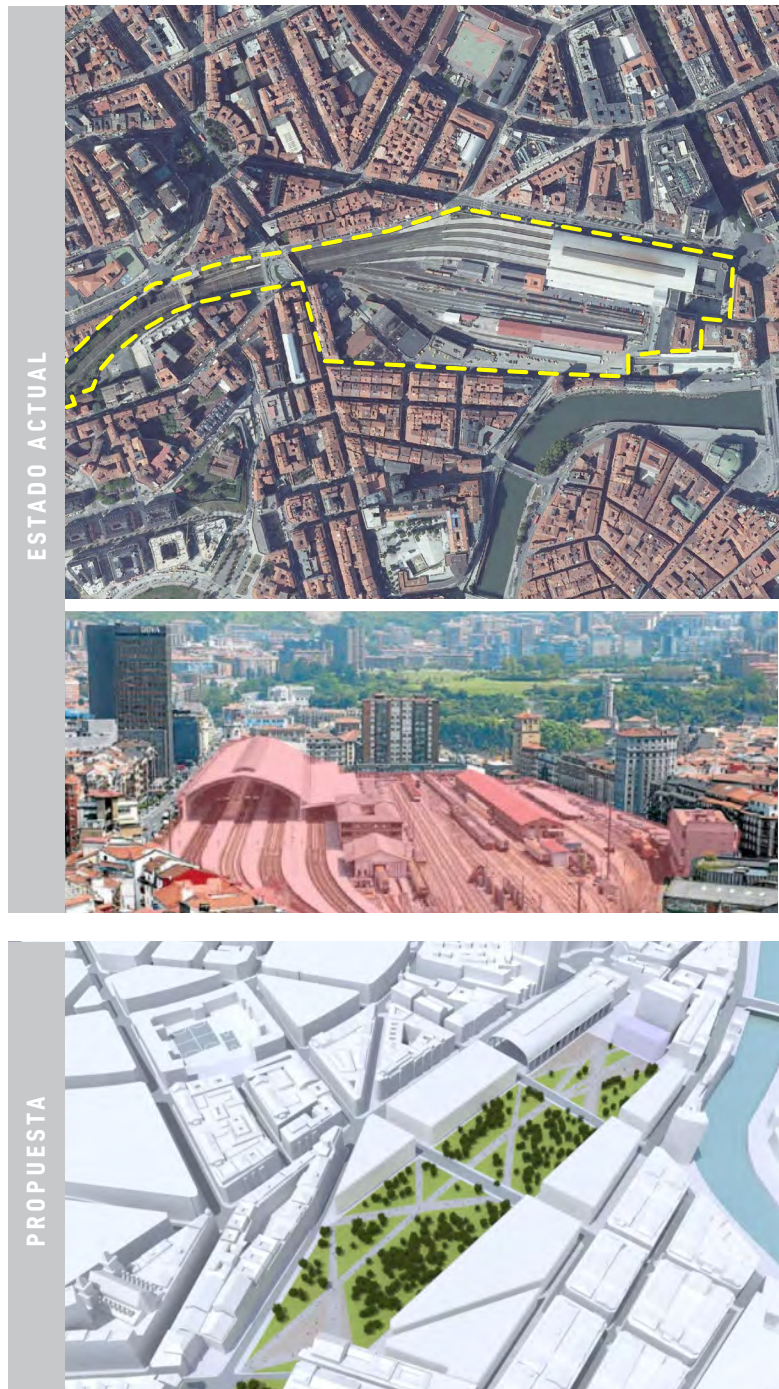
Figure 6.4: Regrading project of the Abando station area: The train lines are moved underground, together with the new high speed line, and the area above is further densified and balanced with a new park. Source: Avance del Plan General de Ordenación Urbana de Bilbao 2016: Resumen de propuestas. Bilbao Udal/Ayuntamiento
