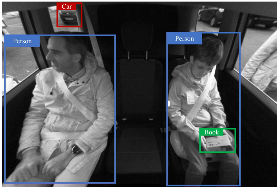
Fig. 1.1 Detected objects inside a vehicle interior by a pre-trained YOLO model. The model detects the people correctly, but it is also affected by objects inside the vehicle (book - which is actually a box of a toy) and outside the vehicle (car).
