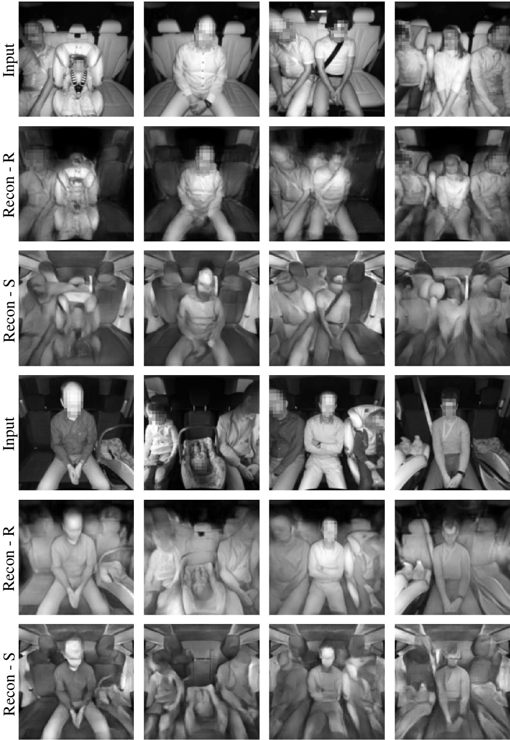
Fig. 6.9 Individual models were trained on real images from an X5 (first row) and Sharan (fourth row) and on synthetic images from the Tesla using the perceptual loss. The models were then applied to real images from the vehicle not used during training. Recon-R are reconstructions when trained on real images and Recon-S when trained on synthetic ones.
