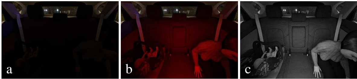
Fig. 3.9 Comparison between a standard RGB image and our simple approach to imitate an active near-infrared camera system for a dark scenery. a) Standard RGB image in environmental illumination. b) RGB image of the scenery illuminated by an active red light. c) Red channel only of the RGB image of the illuminated scenery (used as infrared imitation).
