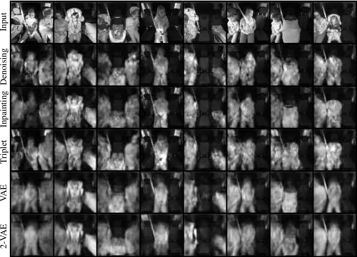
Fig. 2.8 Reconstruction results of ORSS test images (first row) for autoencoder models being trained with different regularization methods (following rows).
