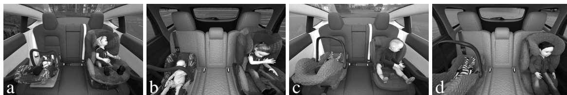
Fig. 6.1 Synthetic images from SVIRO. Left: infant seat with a baby, Right: child seat with a child. Training on images from a single vehicle interior (a): How can we improve robustness on same class instances, but to a new vehicle (b)? Can the model generalize to new class instances in the vehicle it was trained on (c)? How can we improve generalization to new class instances in a new vehicle (d)?
