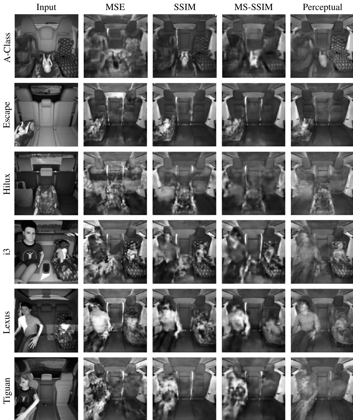
Fig. 6.7 Reconstruction of the same examples as in Fig. 6.6 for autoencoders trained using the nearest neighbor up-sampling instead of max-unpooling with indices. The first column contains input training images from unknown vehicles. The other columns show the corresponding transformations by the autoencoder for different cost functions used: MSE, SSIM, MS-SSIM and perceptual loss. The model was trained on the Tesla vehicle. The results are blurrier and less stable as for max-unpooling.
