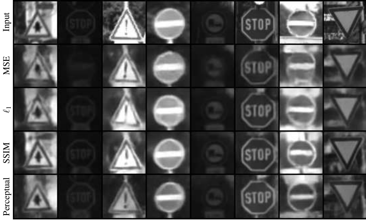
Fig. 2.4 Reconstruction results of GTSRB test images (first row) for autoencoder models being trained with different reconstruction errors (following rows).
