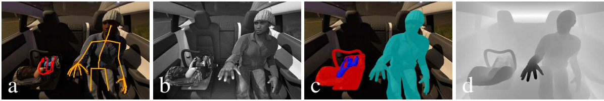
Fig. 3.10 Example scenery of SVIRO together with some of the provided ground truth data. Left seat: infant seat with an infant. Middle seat: empty. Right seat: adult passenger. a) RGB image with keypoints for human pose estimation. b) Grayscale near-infrared imitation. c) Position and class based instance segmentation. d) Depth map.
