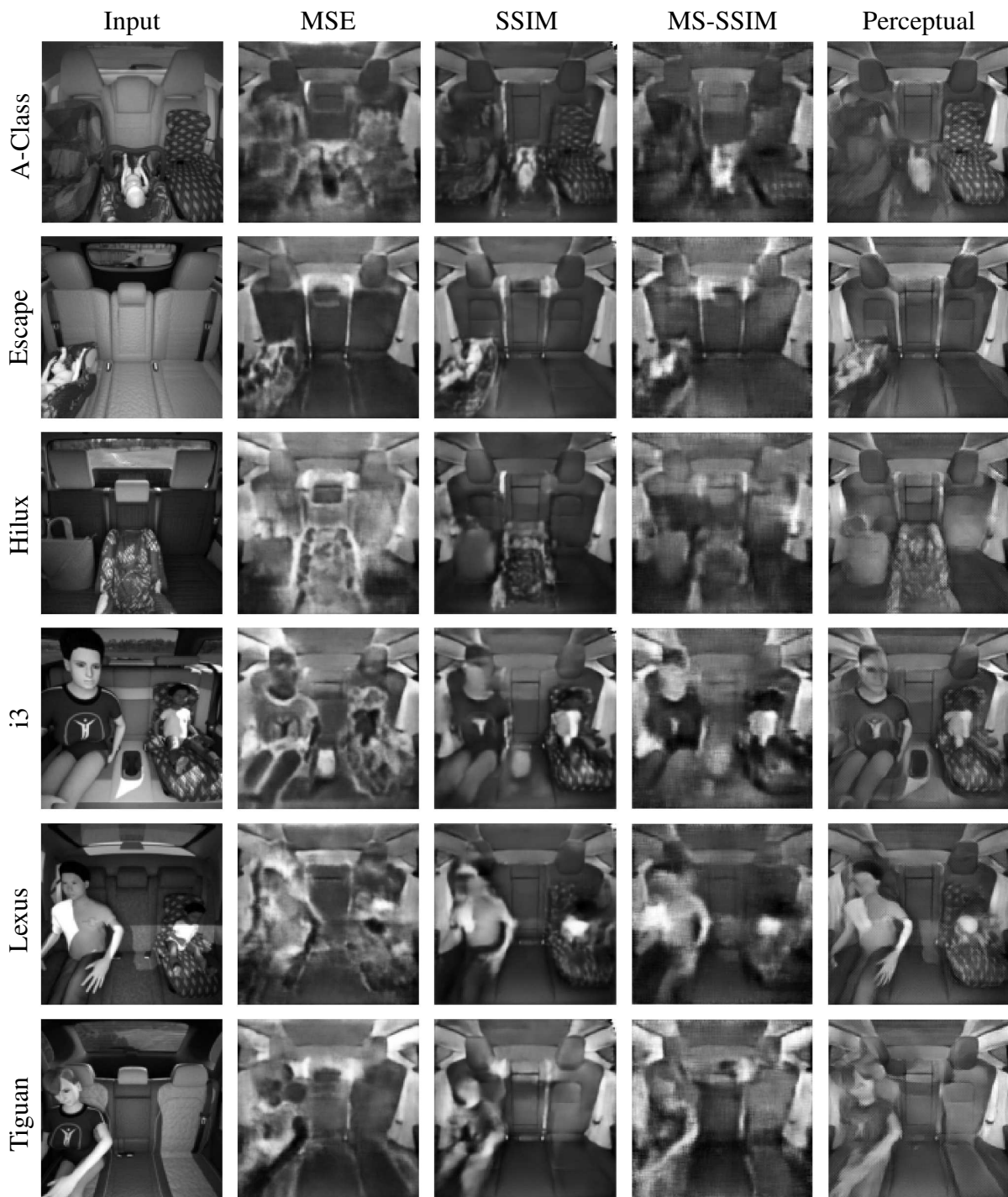
Fig. 6.6 Autoencoders were trained on the Tesla using the de-noising approach. The first column contains input training images from unknown vehicles. The other columns show the corresponding transformations by the autoencoder for different cost functions: MSE, SSIM, MS-SSIM and perceptual loss.
