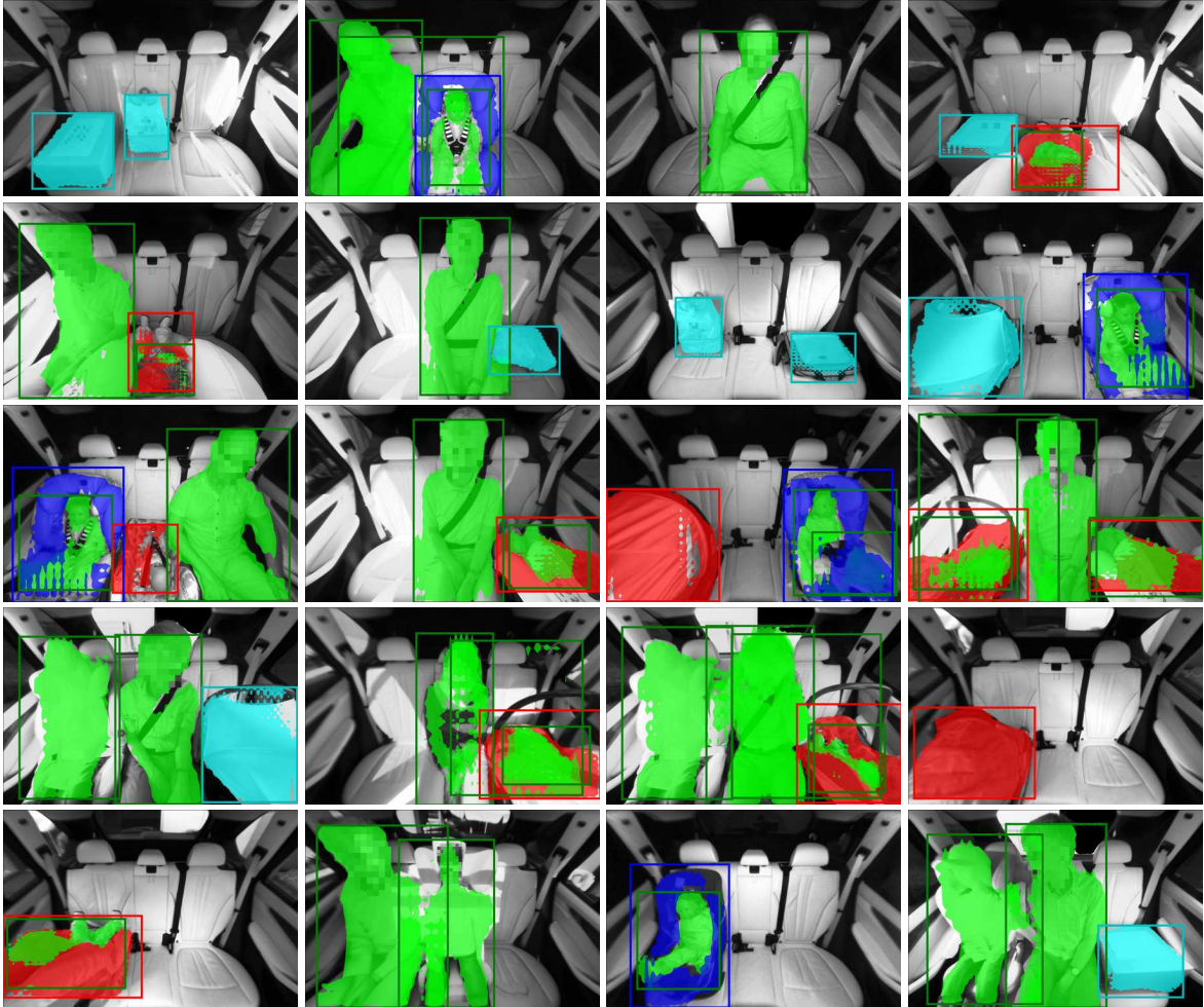
Fig. 5.6 Instance segmentation predictions on real images by a model fine-tuned on SVIRO.
